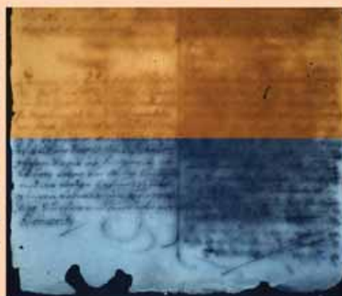
Comparison of readability of text in normal and UV light (blue)
