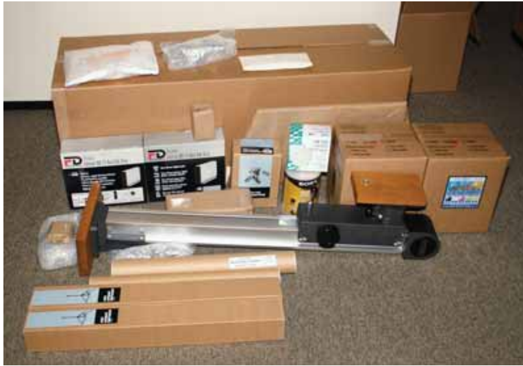
Figure 3. Components of HMML manuscript imaging system ready to pack into oblong shipping box for sending to digitization site. Imaging studio can be shipped in a box measuring 42 x 42 x 120cm.
