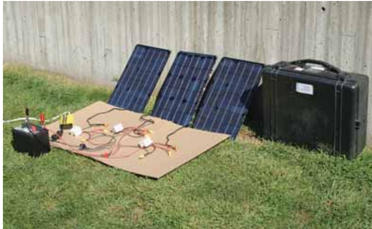
Figure 10. Prototype solar power system for HMML preservation projects in locations without electricity. Three-panel system can power a laptop computer, external hard drive and camera battery charger. Items fit into carrying case for easy transport.
