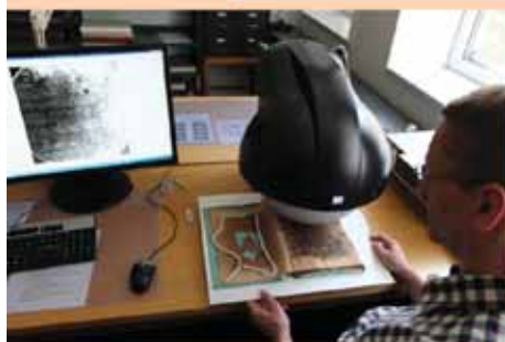
Testing VideometerLab, a danish tool for digital copying, using 18 different predetermined wavelengths of light in UV and NIR range.
